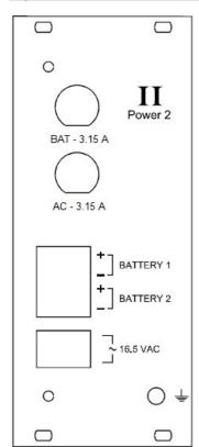
BAT – 3.15 A – Fuse to protect battery circuit.
